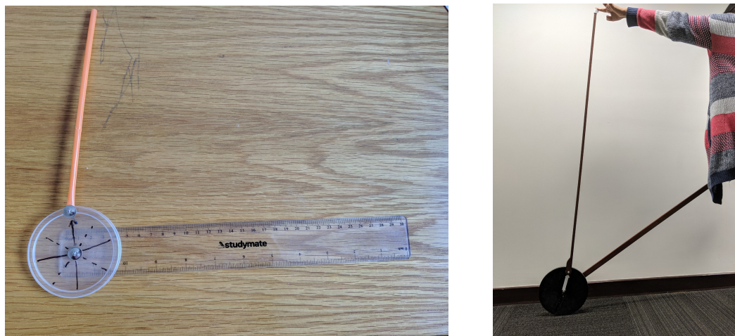
Fig. 2. (Right) Phasor-wheel model. A circular wheel with a handle and an arrow marked on it. A linear stick attached to the wheel makes a sinusoidal wave-like pattern when projected on a wall as it moves forward. (Left). A cup-lid wheel, same as the wooden wheel, can be used to trace different path lengths on an A3 paper.
